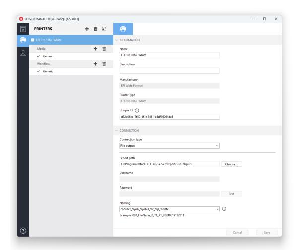
When set up this way, the Fiery XF server RIPs the job and creates a \*.bco file. Use the printer software to select the \*.bco file and print the job.
